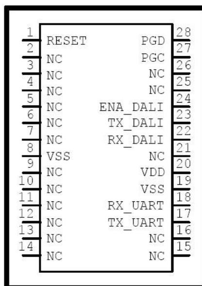
The Dali Bridge chip is able to make an easy interface between a serial uart ttl bus and a Dali bus. With a few command it's possible:
